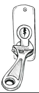
1. Grab the lower part of the lock with the monkey wrench. (if that's imposible because the part of the lock sticking out is too shallow, break off the cover around the lock, by putting a screwdriver or crowbar under it. use force!) Now move the wrench softly left and right a few times, creating some movement. After this, use force and push the wrench to one side, breaking off the front part of the lock.
